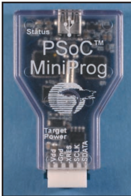
Photo 2 —This little bugger kept my PSoC emulator in the box. I was able to program my CapSense code changes into the CY8C21001 and run them without having to remove the PSoC MiniProg module from the CY3212 CapSense training board's ISSP socket.
