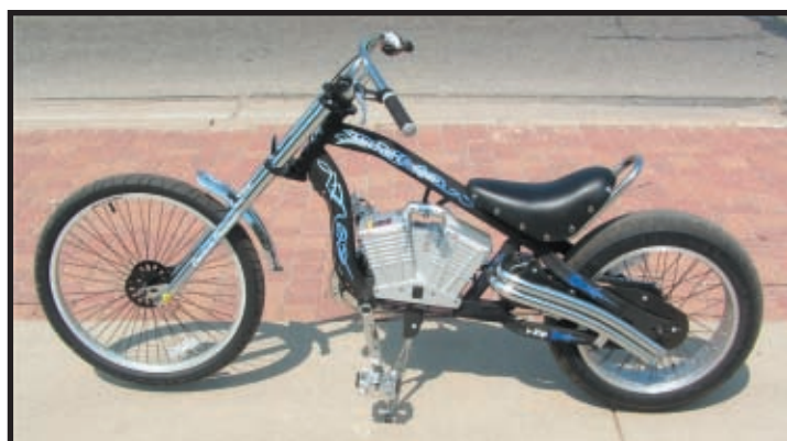
Photo 1 —Currie Technologies produced this bicycle in 2005. It's unusual for a bicycle to be electrically powered right from the get go. It uses twin 12-V, 12-A batteries to power a 350-W DC motor.
