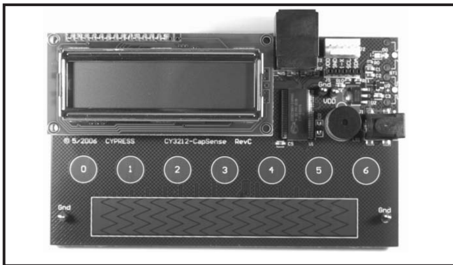
Photo 1 —The CY3212 CapSense training board is very unassuming. There's just enough stuff here to sense your finger on the pads and the slider. The training board includes a CY8C21001 OCD part, which adds a bunch of advanced debugging clout to this unassuming development board.
