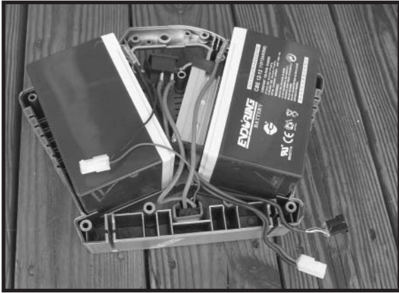
Photo 2 —Cracking open the plastic engine shell reveals two 12-V, 12-A-h gel cells and a solid-state 40-A motor controller. Two external connectors can be seen at the bottom right of the photo. The large high-current connector goes directly to the DC motor and the smaller 1 x 6 plug interfaces to the twist-grip throttle mounted on the right handlebar.
