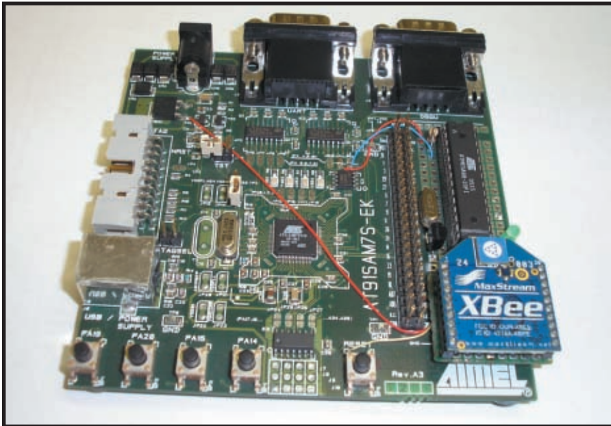
Photo 1 —I modified the AT91SAM7-EK board. I placed the Xbee radio module and the ATmega88 in the DIP package in the prototyping area.
