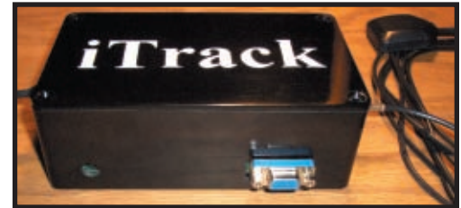
Photo 1—The finished project is housed in protective black Bakelite casing. A cell phone antenna is on the left and a GPS antenna is on the right. Power and serial connectors are in the front.
